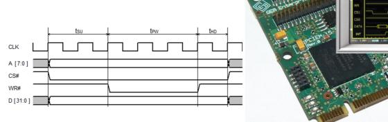
The IOBUS shall be the bus used for communication between a master (the Pcie card) and an unspecified number of slaves. The bus supports up to 32 Data bits, up to 8 bits address, 2 Chip Select (CS#), Read Enable(RD#), Write Strobe (WR#), Interrupt request (INT#) and an optional Wait signal (WAIT#).
