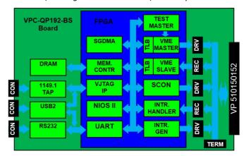
The interrupt handler function is able to read the status of the interrupt lines, making it available to Interrupt read status commands. The interrupt handler can also perform interrupt acknowledge cycles at any IPL level to reset interrupt source and get its vectors.
