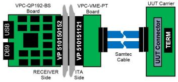
to the impedences will be duty. A standard VME tracks have an impedence of 100 ohm when unloaded, under 50 ohm when full loaded. Using of 50-ohm, high density, shielded cable, like Samtec HQCD, will be a good idea. A transition board named VPC-VME-PT can be supplied on request.
