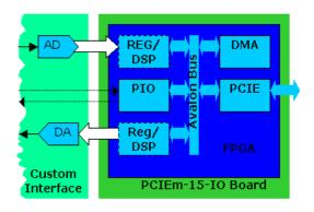
**PCIOM-15-10** Mini-PCIe size, The best and cheapest solution for systems on box allows the user to control electrical interfaces of your SBC to external I/O resources (i.e. motors, transducers, sensor, CCD and so on). Altera Fpga provides the user with up to 53 general purpose I/O and 3 dedicated Clocks with PLL, and up to 2Mbytes of on board SRAM, and a FPGA with about 15KLE (400Kgates) or 30KLE (800Kgates) resources. The JTAG connector allows the ISP programming using an ALTERA USB blaster.
